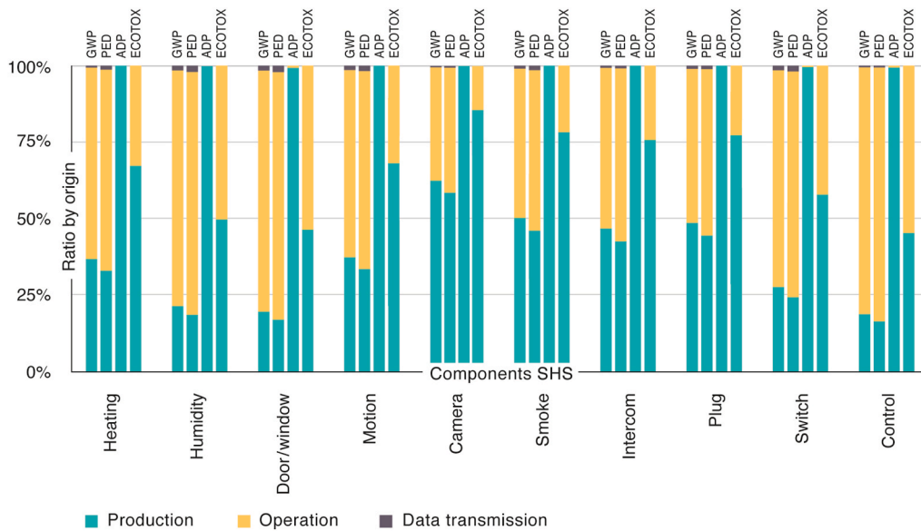
Fig. 6. Relative share of GWP, PED, ADP and Ecotox of the SHS for production, operation and data transmission over life time.
